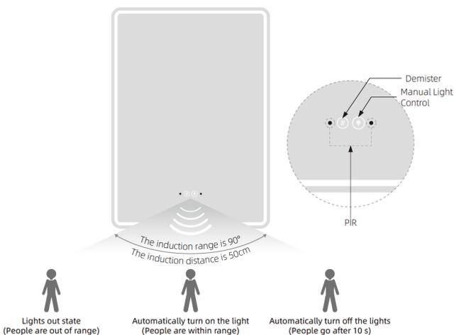
Activate the mirror by just walking into the room! Part of our automated bathroom solutions, our PIR sensor knows exactly when you need the lights to turn on and it activates the mirror automatically by gently lighting up the room, this comes specially useful at night when it's harder to find the switches.
